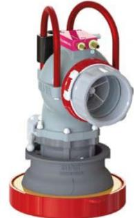
The Model 353GF Pressure Control Coupler is a hydrant coupler used in jet aircraft refuelling operations. It connects to a hydrant pit valve or hydrant pit adapter to allow pressurized fuel to flow from an underground pipeline and into the receiving aircraft. It incorporates a Deadman operated, direct acting pressure regulator that protects the receiving aircraft from excess pressure and from damage due to pressure surges.
