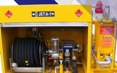
Fuel Sampling Jar, 3.5 Litre Sampling Jar to check for Water and Particles in the Fuel
