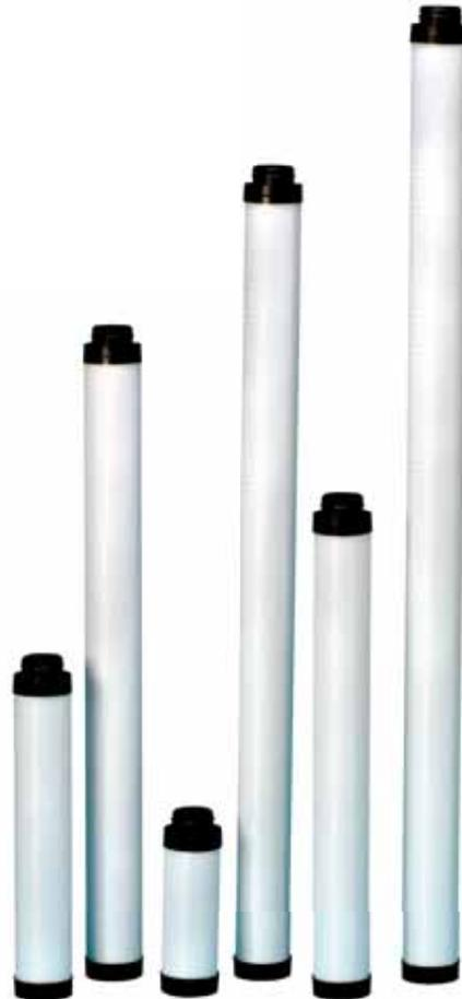
As the cartridge removes water and/or contaminant from the influent fuel the pressure differential will increase along with a decrease in flow rate. These changes are the result of flow restriction caused by dirt retention or water absorption in the media. The rate of these changes depends on the quantity of water or contamination in the fuel.
