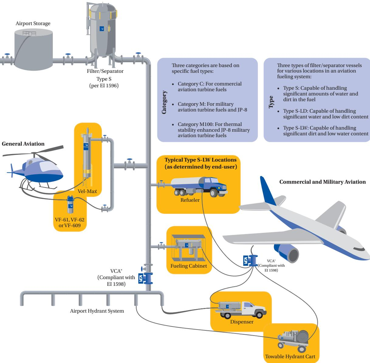
\* Prefilter elements compliance with EI 1590 and vessel compliance with EI 1596 is customer dependent. Optional EI 1583 Qualified Vessels/Absorbent Type Cartridges for jet fuel without anti-icing additive.
