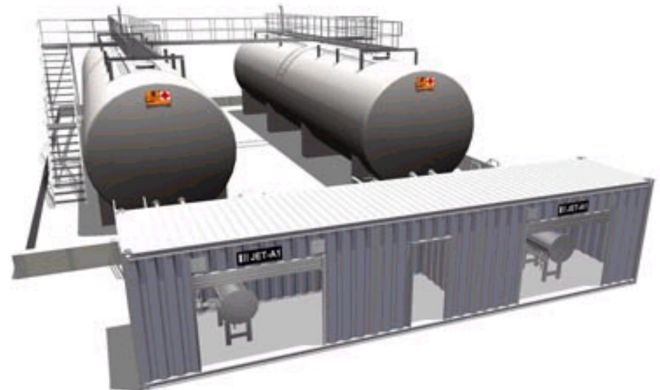
FUEL FARM / HORIZONTAL TANKS
