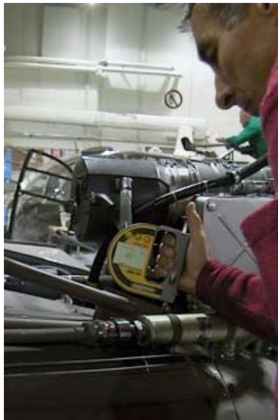
Fig.1 Filling sample from the oil container
